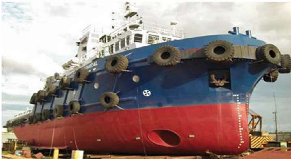
Completed Anchor Handling Tug Supply Vessel waiting to be launched
